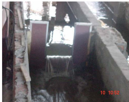
Figure (4): Rectangular weir.
